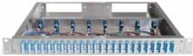
Compact, pre-assembled FO-DCS 19"/1U panel, version with 8 MTP couplers (rear) and 48 OM3 LCD ports turquoise (front)
