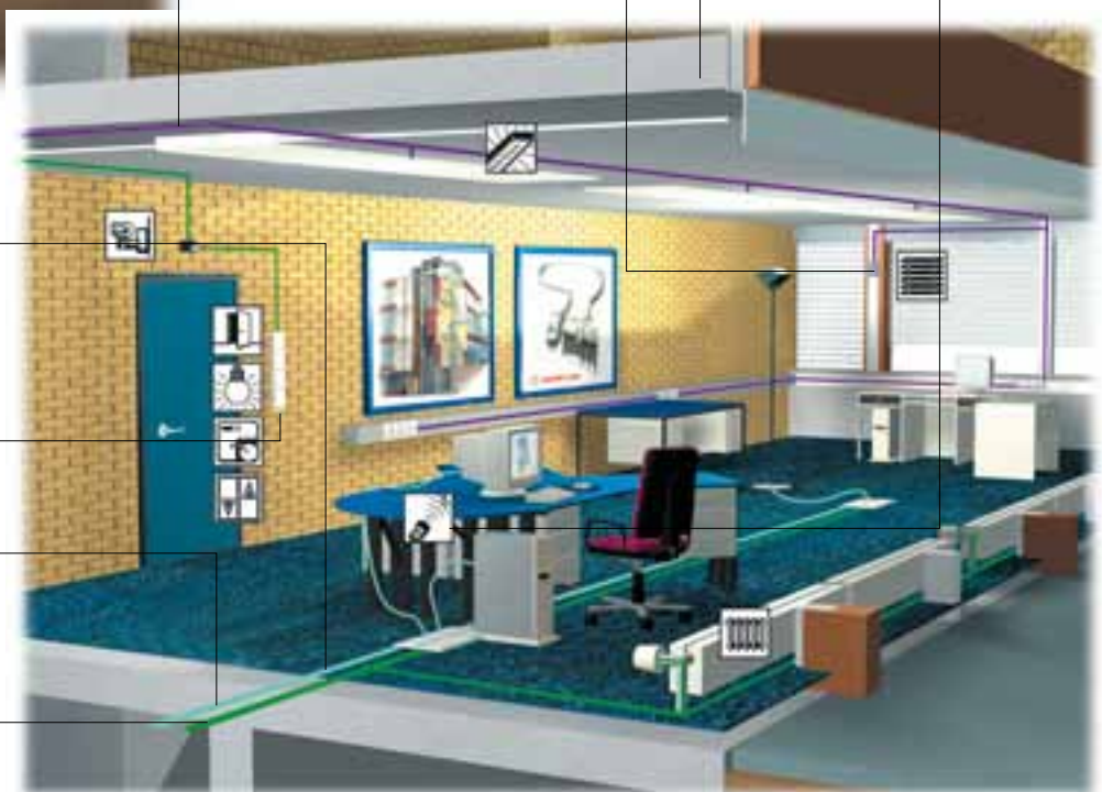
Platform cable Power 5x10 with Power 5x10 Adapter out power output circuit for flatform cable Power 5x10mm 2 e.g. pre-assembled with floor boxes and output circuit fuse
